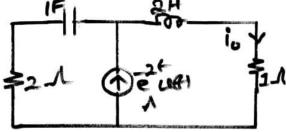
b) Determine the current *i* for  $t \ge 0$  if the initial current i(0) = 1 for the circuit [7M] shown below by Laplace transform.
